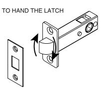
Remove forend plate and rotate the latch head. Replace forend plate.
