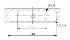
\* Optional drilling for security locking with M4 grub screw. For details refer to Triade maxi instruction sheet. [4]
